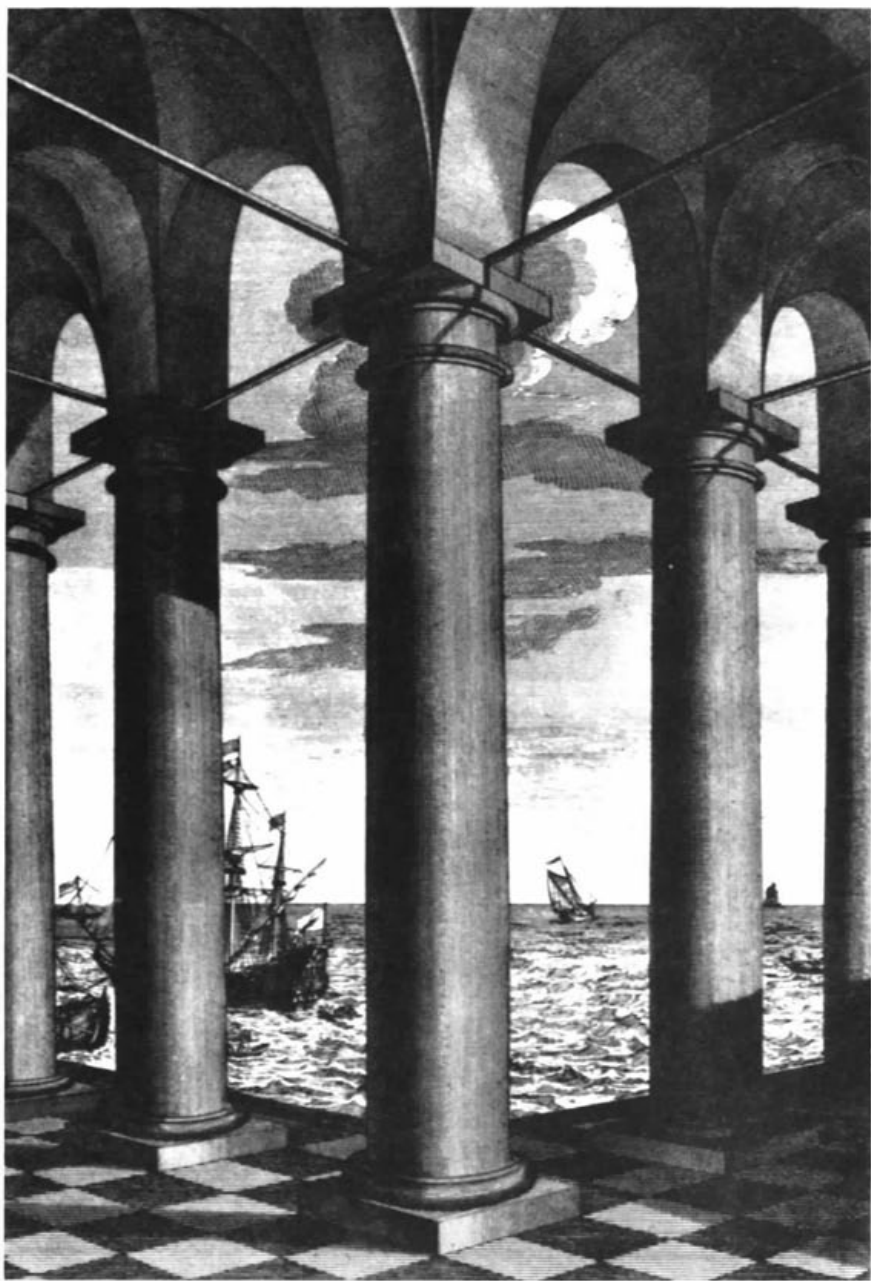
Cambered (transverse) vaults and metal tie-beams. From Leone Battista Alberti, Ten Books on Architecture , translated into Italian by Cosimo Bartoli and into English by James Leoni (London, 1755), plate 9
