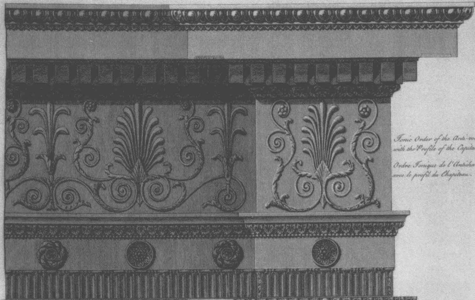
Cornice & Base of the Architrave over the Columns.
