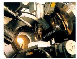
The X-ray diffractometer plays a key role for the Gallery's scientists and conservators in the analysis and characterization of crystalline materials
