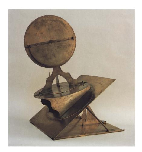
in it is a second recess for plates. These include a plate for latitude 48° and another of the twelve astrological houses. A small magnetic compass is inset in the front of the suspension-piece; this is an unusually early example of such practice.
