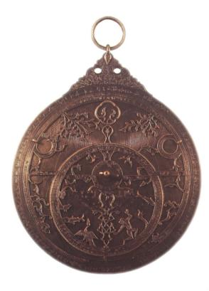
stars around the North Pole. On the reverse of the *mater* is fixed the alidade, a flat ruler that turns around the pole and which serves to set the instrument and read off the altitude of the stars.
