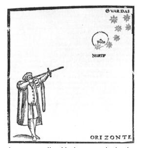
fig. 4. Cross-staff used for determining the altitude of the Polestar, when the Guards are in a particular position. From Pedro de Medina, *Regimiento de navegación* (Seville, 1563), fol. 36
