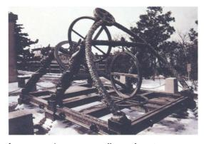
fig. 4. Guo Shoujing's Armillary Sphere (*jian-yi*, "simplified instrument") of 1276, in an exact copy made for the Ming Astronomical Bureau in 1437. Cast in bronze, it measures roughly 12' x 18'; the largest of the rings is 6' in diameter. Photograph courtesy Thatcher Dean, Seattle.
