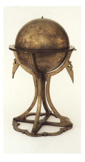
The brass stand, piece-cast and with an applied copper ring, is also graduated but is a later replacement. It is held together below the base by a half-melon shaped screw with a loop below, probably for a plumb-line. J.M.R.
