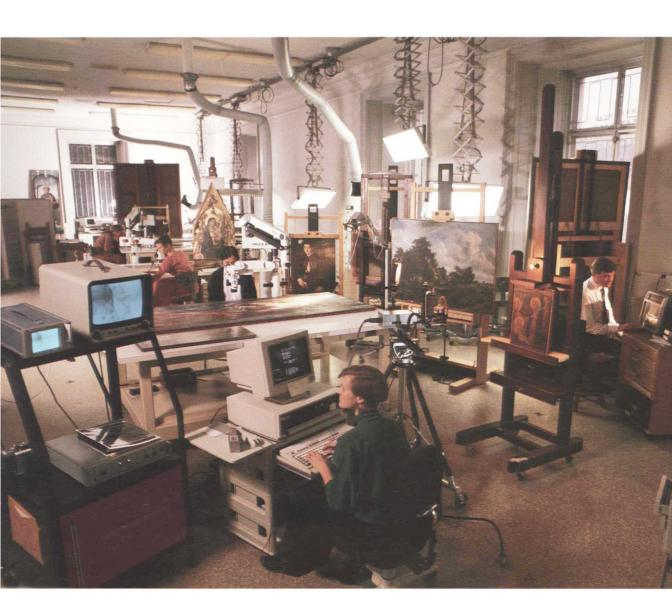
The painting conservation lab. Center, a conservator makes an infrared reflectogram of a painting with camera and computer (page 19). Behind her, conservators examine paintings with microscopes, treat paintings, and study slides of works of art.
