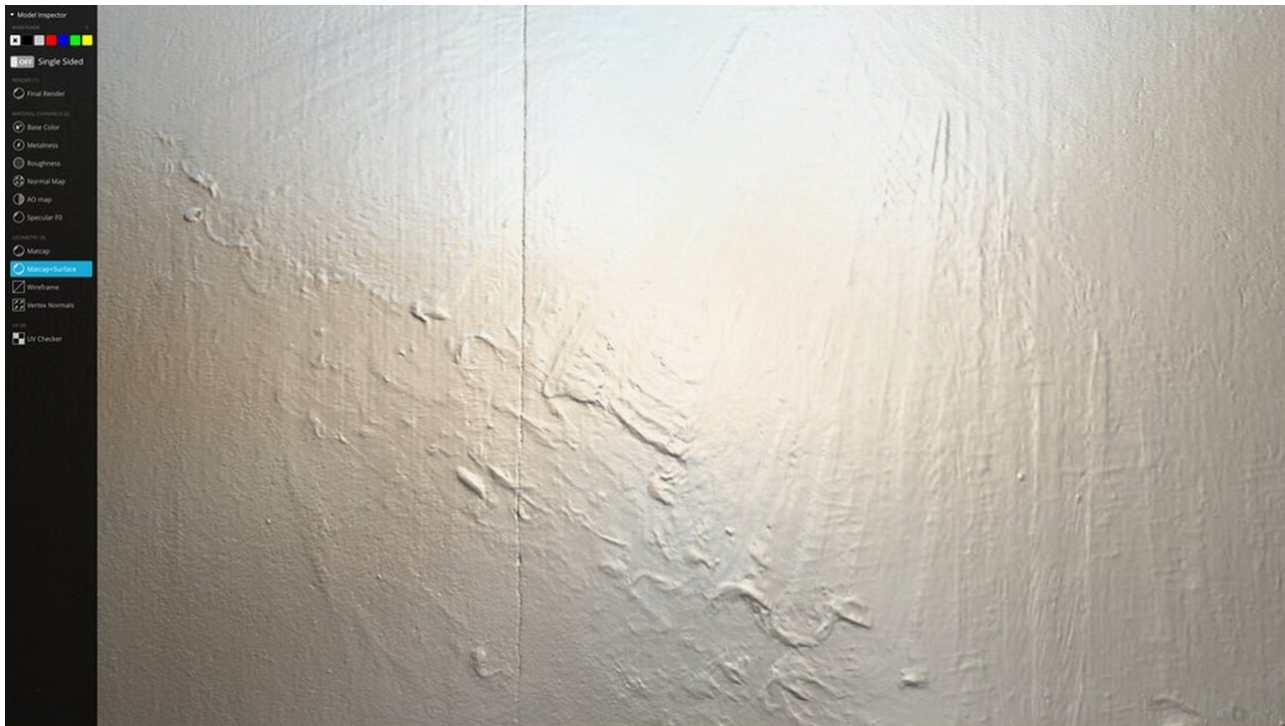
Fig. 5b. Sketchfab web viewer: the same geometry with a surface normal texture applied to allow lighting to highlight the fine details.
