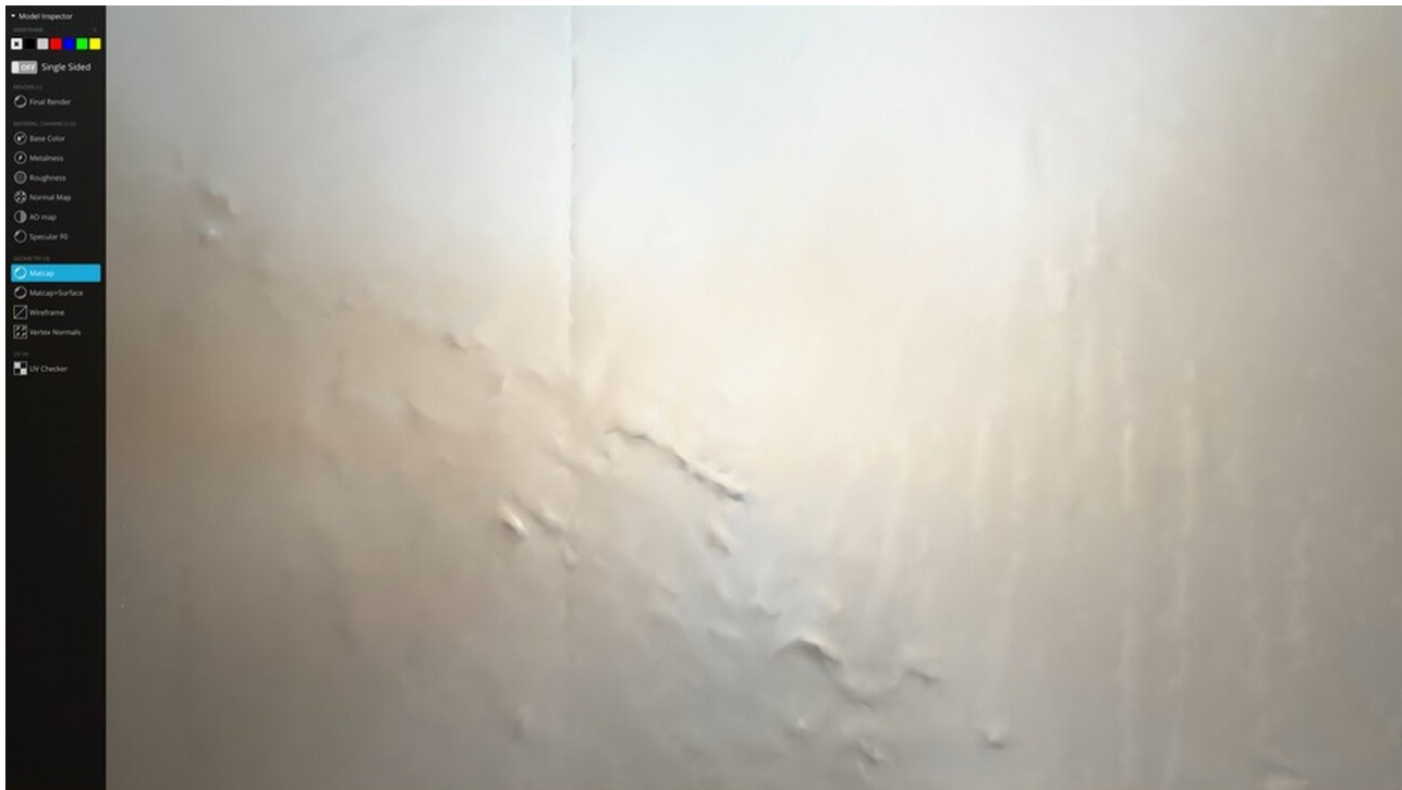
Fig. 5a. Sketchfab web viewer: low-resolution geometry with surface normal disabled, showing lack of fine detail.
