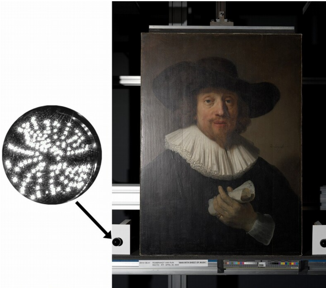
Fig. 2. One image from the RTI capture set. Inset is a composite image of a black sphere showing all of the lighting positions used to compute the reflectance transformation imaging.
