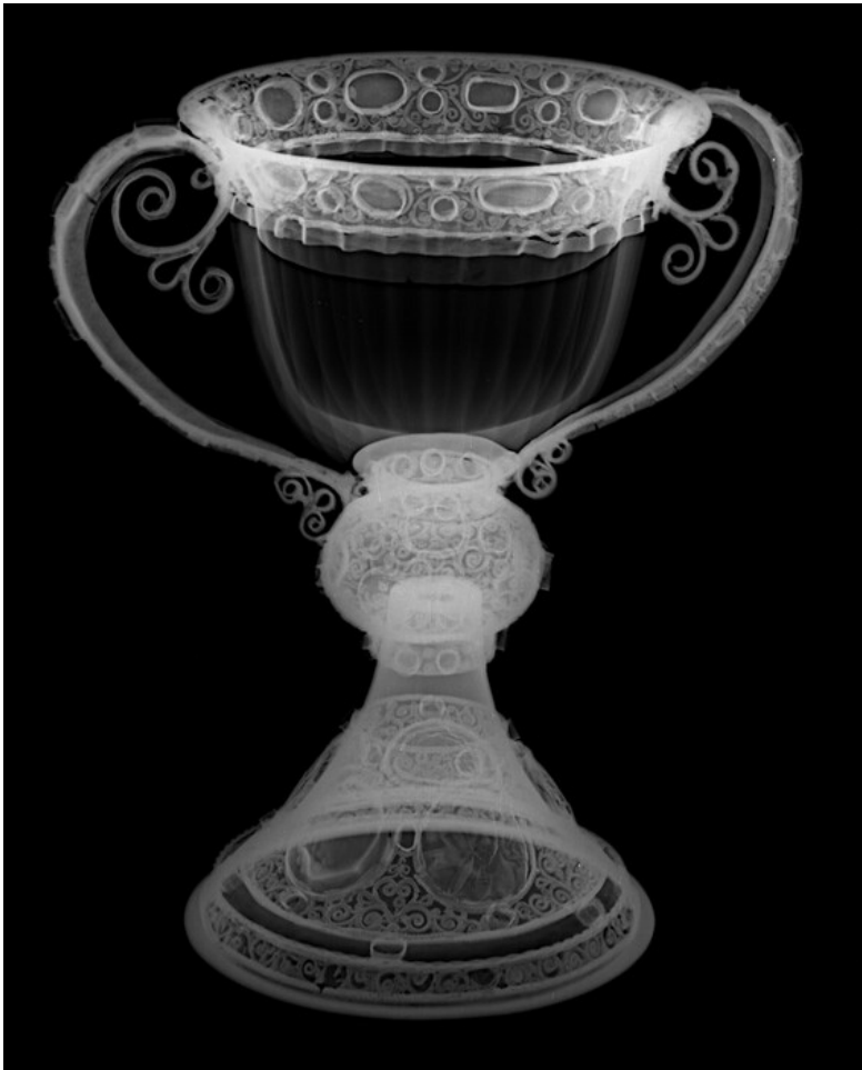
Fig. 20. X-radiograph of Suger Chalice (fig. 1).
