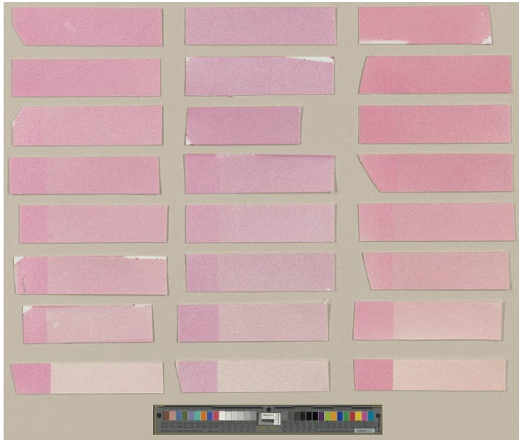
Fig. 16. Cochineal carmine prepared using three different recipes. The left column is un-laked carmine, the center is alum-laked, and right column is tin-laked. The pigment swatches were applied to gelatin-rosin paper and then underwent accelerated aging through exposure to intense light. From top to bottom within each column, the swatches were exposed for 1, 3, 6, 9, 11, 19, 30, and 70 hours. Adapted from Strumfels and Berrie 2017.
